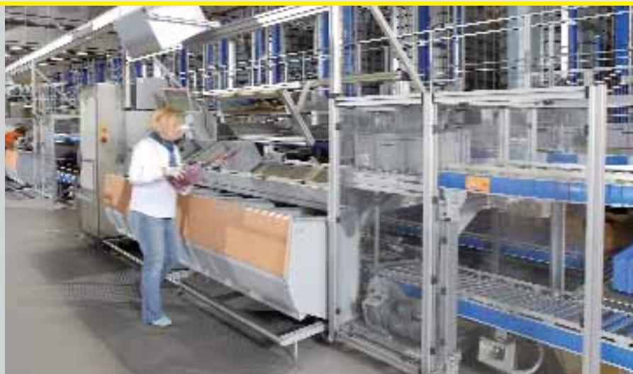
Ergonomically designed workstations: In the SCS goods retrieved from the presented totes are picked downward into boxes for shipping.
